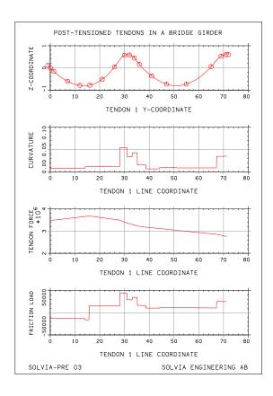
Post-tensioning of tendons in beams can be specified using nonuniform B-splines for the 2D or 3D tendon geometry. One or both of the ends of each tendon can be tensioned in a sequence of applied end forces and length changes from anchorage set. The curvature and wobble frictional losses are calculated and the resulting friction and pressure loads from the tendon as well as the end forces are applied to the BEAM elements.
