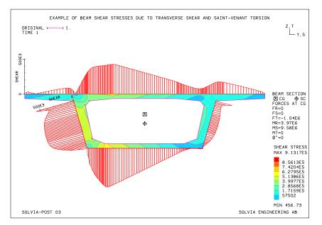
This is an example of a bridge analyzed with a BEAM element model and the new capability T-BEAMSTRESS. The plot shows the distribution of shear stresses over the cross-section due to a set of calculated forces and moments obtained from the BEAM element model. The new option of plotting XY-diagrams in the mesh of the model is also shown.
